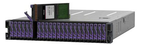
around for storage as it is built to support Western Digital's new Ultrastar DC SN840 NVMe SSDs allowing it to deliver an impressive maximum capacity of 368TB.
